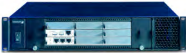
Fig. 3. High cost factor removed: Powerbridge replaced the MicroTCA carrier hub with individual support modules.
